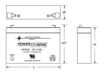
L: 5.24 (133) W: 1.30 (33) **H**: 3.82 (97) Tolerances are +/- 0.04 in. (+/- 1mm) and +/- 0.08 in. (+/- 2mm) for height dimensions. All data subject to change without notice.
